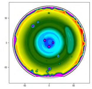
Quality, Uniformity And Defect (QUAD) mapping of a standard epiwafer based on surface voltage differences. Concentric doping and thickness profiles can be seen as well as extended defects (spots) and the substrate's facet. © Fraunhofer IISB
