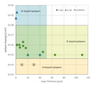
Doping vs. thickness diagram with epitaxial process windows for n-type, p-type and nominally undoped epilayers. © Fraunhofer IISB
