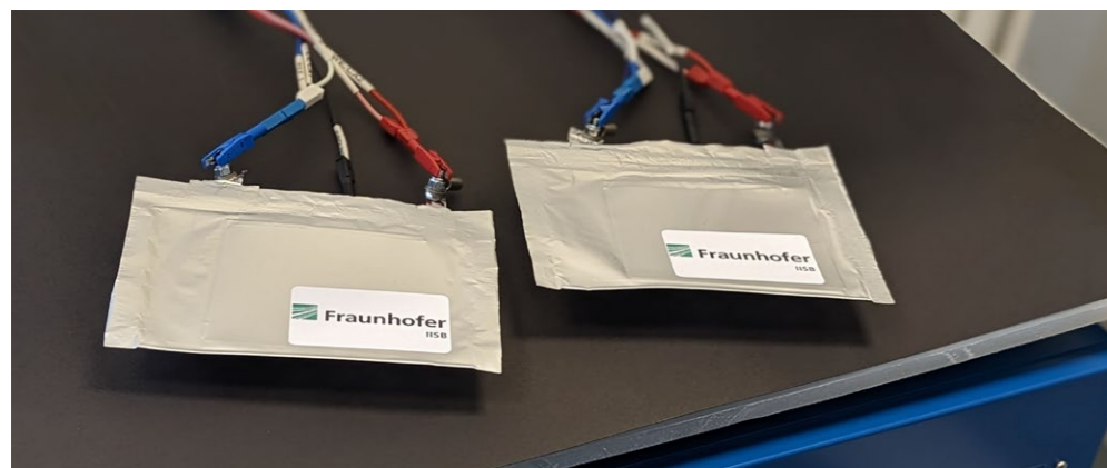
Prototypes for aluminum-ion pouch cells, developed at Fraunhofer THM in Freiberg © Martin Eckert / Fraunhofer IISB
