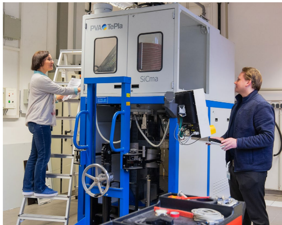
Installation of a PVT (Physical Vapor Transport) reactor suitable for AlN crystals of 4 inches and larger © Elisabeth Iglhaut / Fraunhofer IISB
