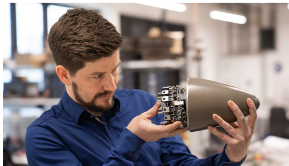
Deep mechatronic system integration enables system advantages - like on this 15 kW multiphase inverter, fully integrated in the aerodynamic nosecone of an electric motor nacelle © Elisabeth Iglhaut / Fraunhofer IISB
