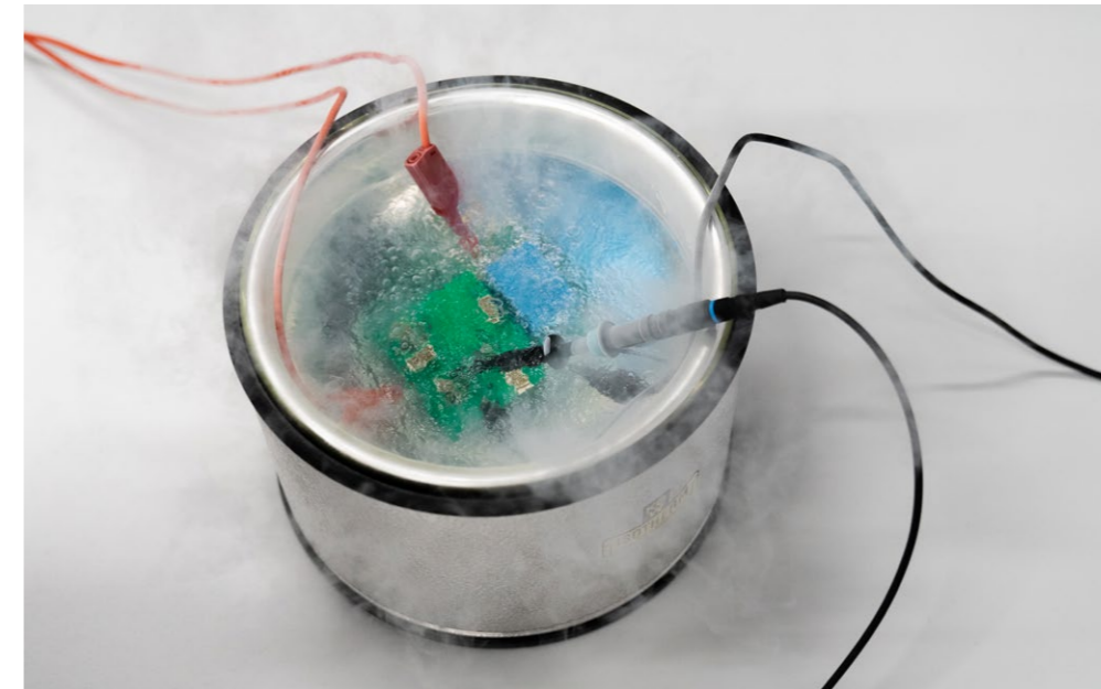
Test of a GaN half bridge in liquid nitrogen © Elisabeth Iglhaut / Fraunhofer IISB
