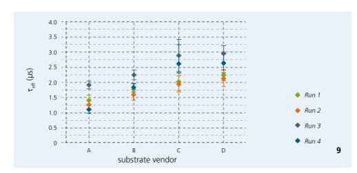
Our efforts show that today's multi-wafer reactors are capable of providing excellent homogeneities and reproducibility with regard to temperature, epiwafer thickness and doping uniformity. This enables engineers to control intrinsic point defects, such as the carbon vacancy. However, the control of some extended defects, or some influences on the effective lifetime are governed by the substrate.
