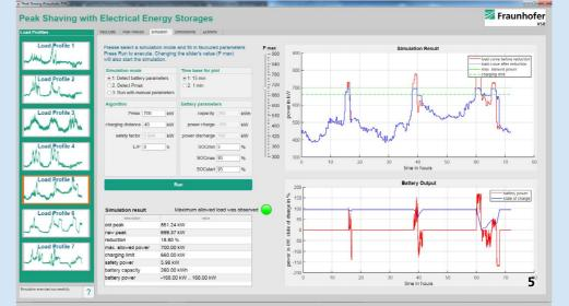
no risk that a peak could happen, the battery system can be charged. To avoid the generation of new peaks because of charging the electrical energy storage, a dead band (charging distance) is introduced. The resulting threshold is called charging limit.
