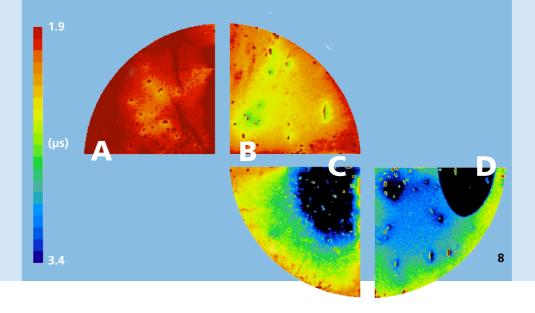
The most common method for determining carrier lifetime is the microwave-detected photoconductivity decay. This method yields a value for the lifetime that depends on the Shockley-Read-Hall lifetime of the epilayer itself, but also contains contributions related to surface recombination and interface effects between the epilayer and the substrate. The value for this effective lifetime is always less than that for the Shockley-Read-Hall lifetime of the epilayer.
