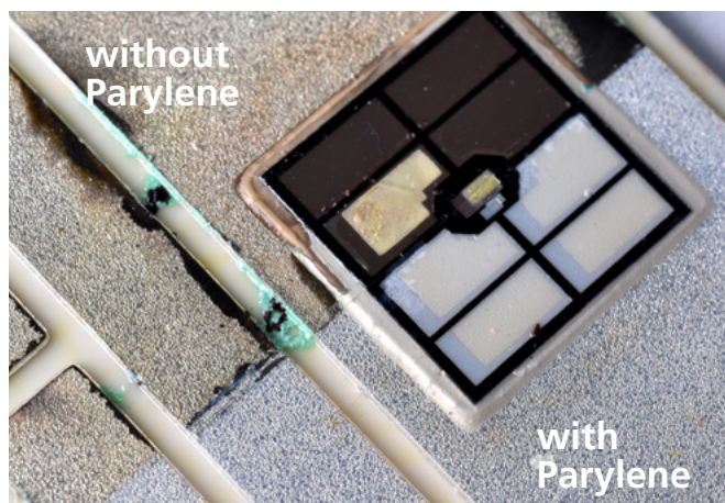
Protection against corrosion by Parylene coating: AMB circuit carrier after exposure to hydrochloric acid © Antonia Diepgen Fraunhofer IISB
