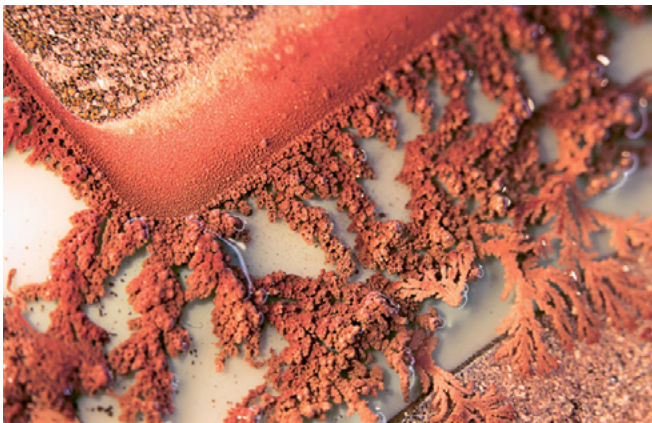
Dendrite formation on a ceramic circuit carrier caused by ECM © Anja Grabinger / Fraunhofer IISB
