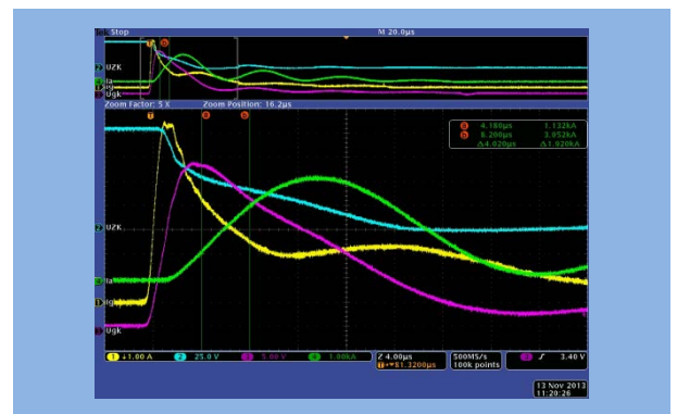
Switching behavior check on power semiconductors
